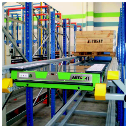
Satellite Storage System
