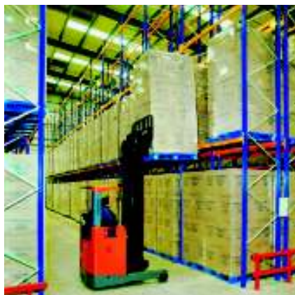
Wide Aisle Pallet Racking
